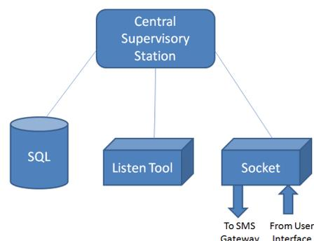
Figure 2. Central Supervisory Station Components
