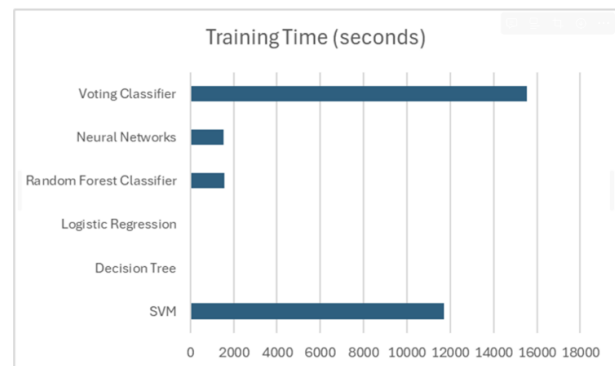
Figure 5. Time needed for models to train on the incomplete dataset.
