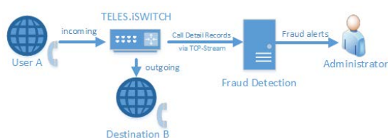
Figure 1. Depiction of the generation of call detail records and a detection system using them.
