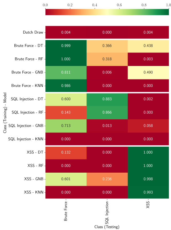
Figure 3. Experiment 2 average F_1 scores for the CIC-IDS-2018 to detect known and novel Web attacks.
