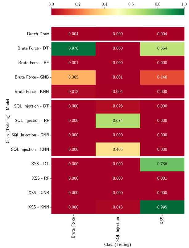
Figure 6. Experiment 2 F_1 average classifier scores when trained on the CIC-IDS-2017 Web attacks and tested whether they were able to detect CIC-IDS-2018 Web attacks.
