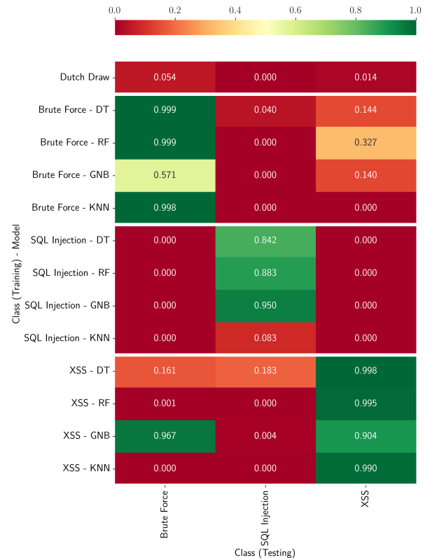
Figure 2. Experiment 2 average F_1 scores for the CIC-IDS-2017 to detect known and novel Web attacks.
