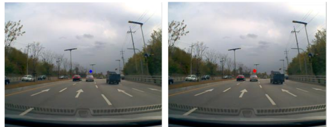
(a) No scaling (b) 1/4 scaling Figure 4. Detected vanishing point with different scaling factors of the voting map.
