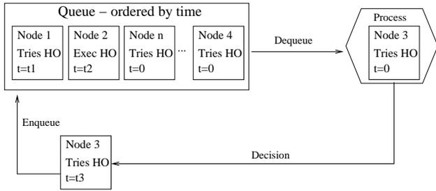
Figure 9. Example of scheduler instance in our discrete-event simulator.
