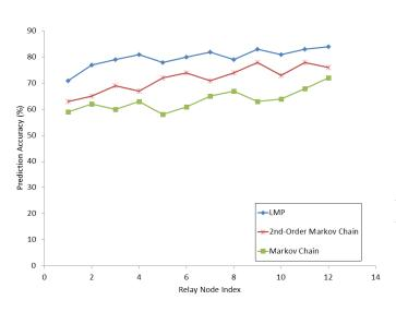
Fig. 6. Comparison of prediction accuracy for the proposed LMP algorithm, generic Markov chain and second-order Markov chain for User Node 2 in networks with 120 users, 14 relay nodes and 1 base station
