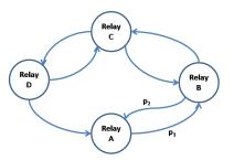
Fig. 3. Example to show a simple Markov chain that depicts the transitions of a mobile user to various relay nodes
