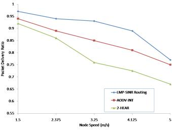
Fig. 7. Packet delivery ratio versus varying node speeds for T = 10ms
