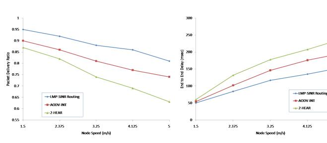
Fig. 8. Packet delivery ratio versus varying node speeds for T = 1ms
