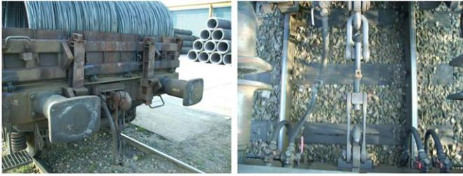
Figure 1. Freight carriage connection
