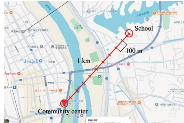
Figure 8. Location map of transmitter- and receiver-side nodes
