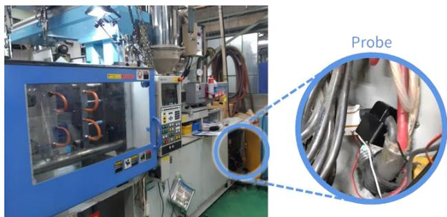
Figure 16. Overview of the field test. The fabricated probes and circuit were applied to the injection molding machine.
