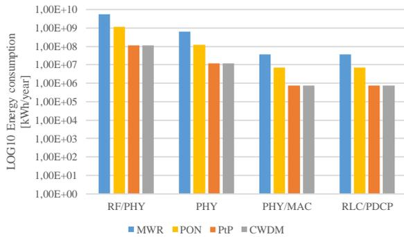
Figure 11. 5G FH energy consumption for different FH technologies.
