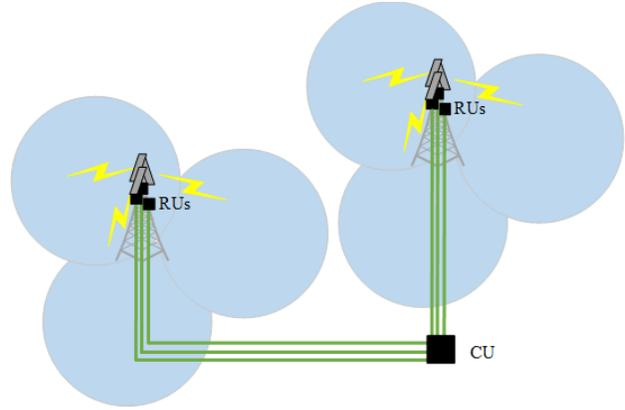
Figure 9. Illustration of several RUs connected to the same CU.
