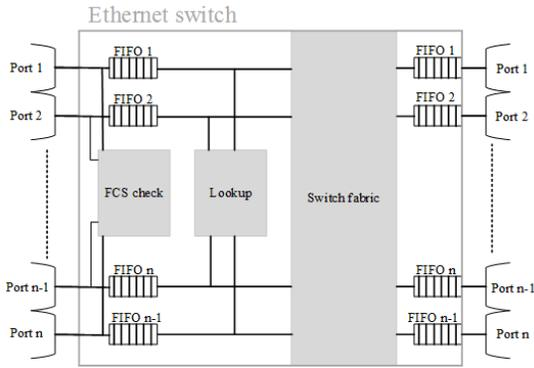
Figure 12. The construction of an Ethernet switch
