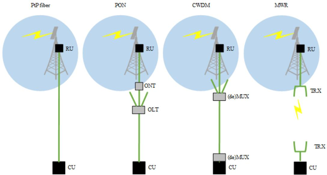
Figure 3. Illustration of different solutions for FH transport technologies: PtP, PON, CWDM and MWR
