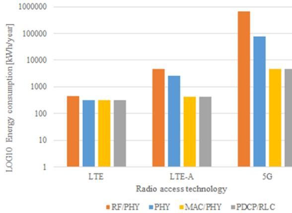
Figure 15. Ethernet energy consumption by radio access technology.
