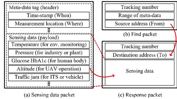
Figure 2. Structure of the sensing data, find, and response packets.
