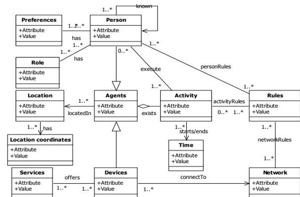
Figure 6. The proposed class diagram.
