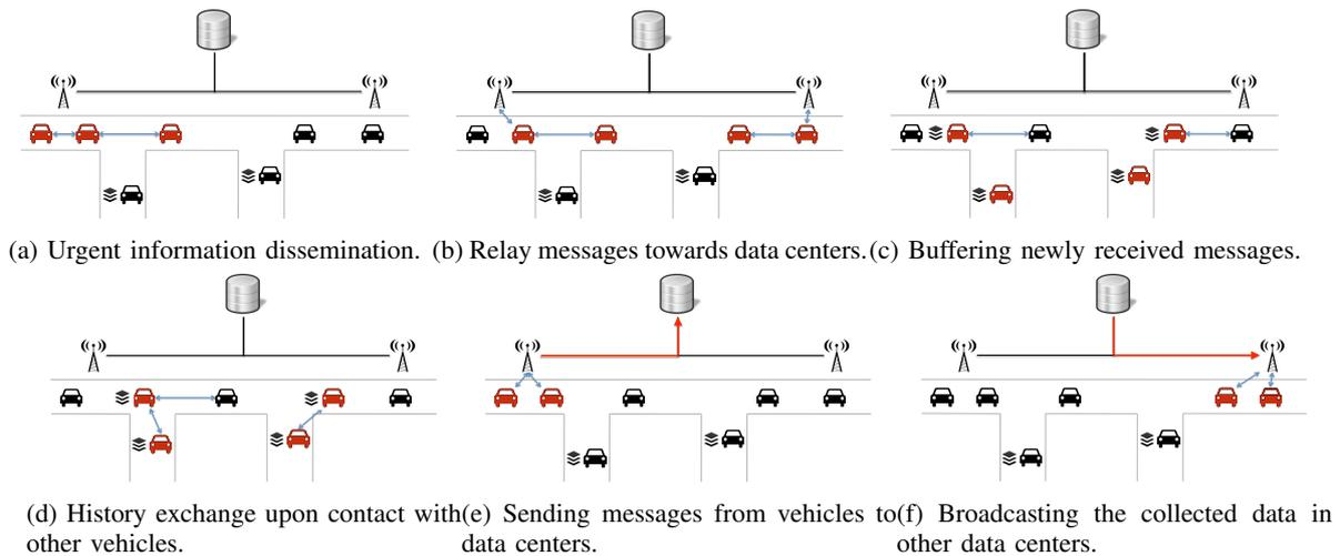
Figure 2. The combination of V2V, V2I and DTN communication model used in VVID architecture.
