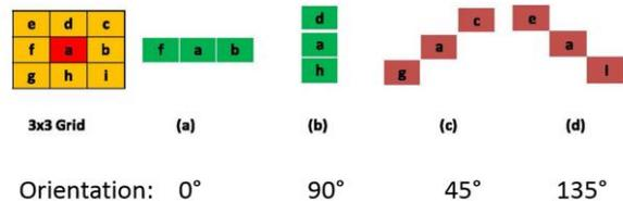
Figure 1. 3-element vector extraction [11]
