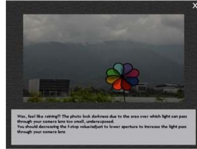
Figure 12. An example of bad settings (too dark) of aperture F/22 and shutter speed 1/1000.
