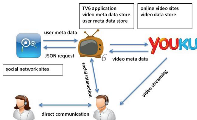
Figure 1. Overview of system architecture
