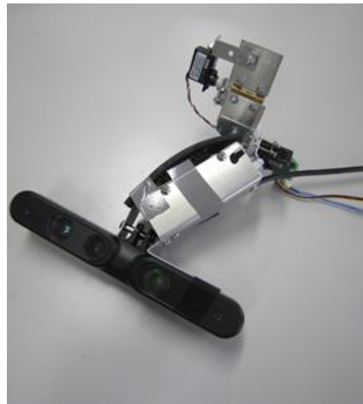
Figure 11. Prototype of FB-Finger2, designed with 2-degrees-of-freedom.
