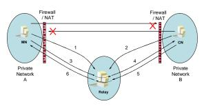
Figure 2: The data relay allows the undirected communication between two nodes behind different firewalls or NAT systems.
