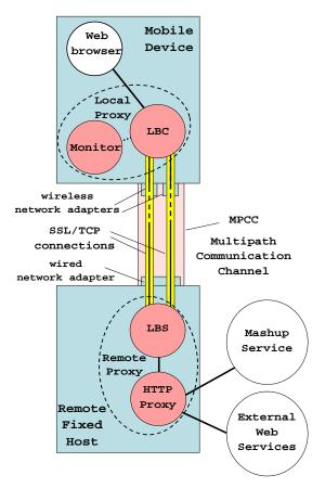
**Figure 5: Architecture for Seamless Navigation**
