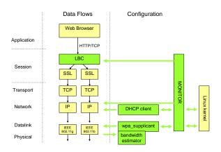
**Figure 6: Mobile Device Software Architecture**
