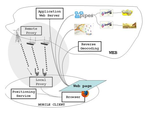
**Figure 3: System Architecture**
