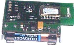
**Fig. 16. ZigBee-ready Temperature Sensor Node**
