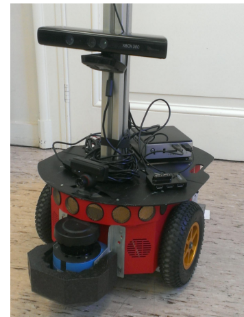
Figure 7. The mobile Pioneer-3dx robot with a mounted Microsoft Kinect Camera, Laser scanner and Sonar sensor.
