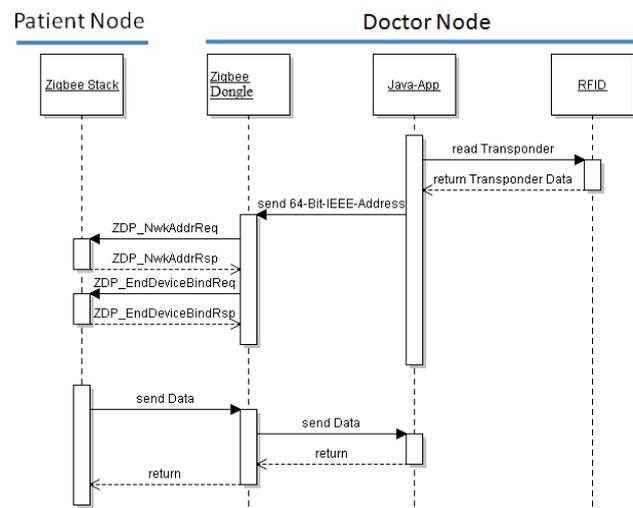
Figure 3. Communication flow diagram of ZigBee-RFID based self-configuring mechanism
