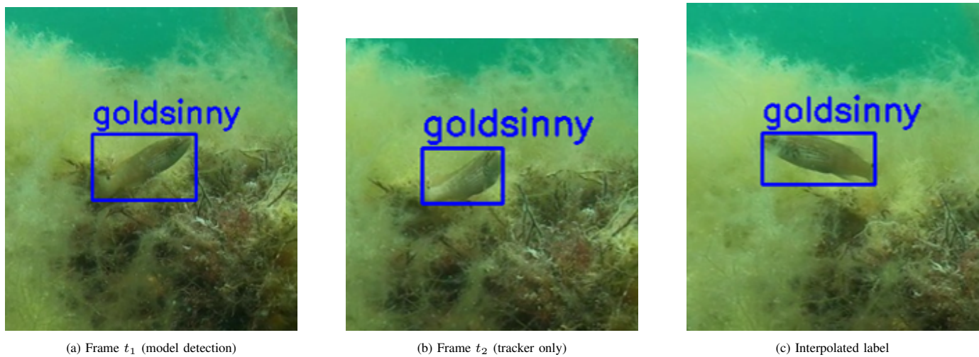
Figure 6. Interpolated pseudolabel generation in practice. Note that due to ByteTrack's use of very low confidence predictions for interpolation, the inferred bounding box does not correspond exactly to the average of the two detections.
