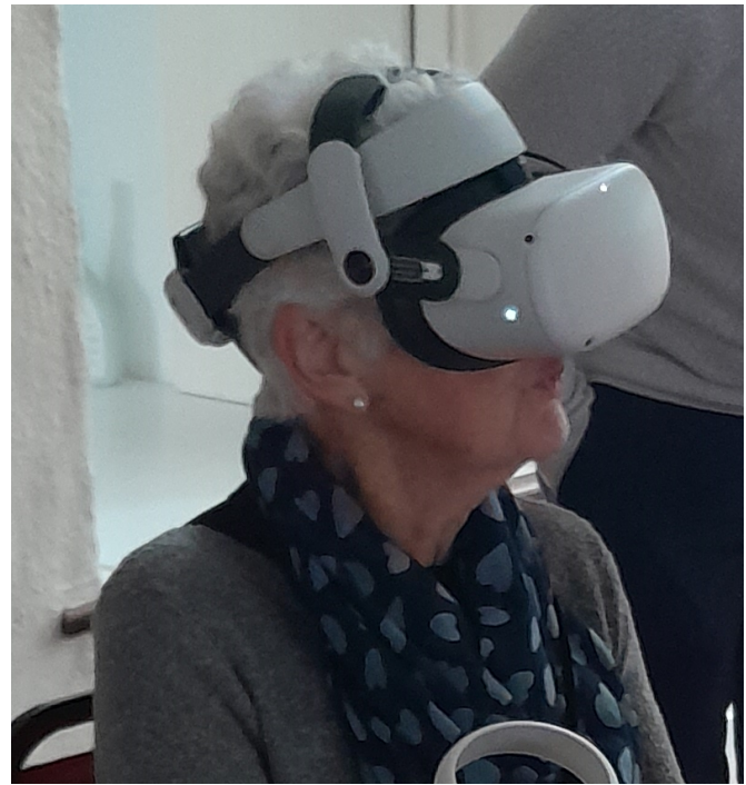
Figure 7. We replaced the original elasticated strap for the headset with a more mechanical strap that distributes the weight of the VR headset equally.
