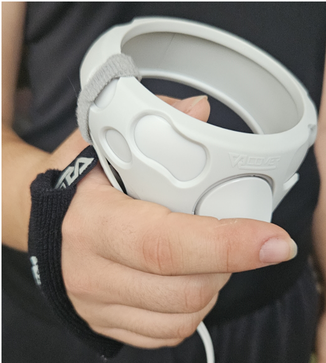
Figure 8. The controller has a strap attached to it that allows the user to open their hand and the controller will stay attached, minimising the amount of strain on the hand.
