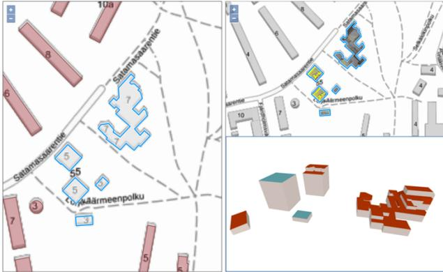
Figure 3. Buildings with on-the-fly computed LOD1 models (bluish roofs), shown together with buildings represented with a pre-created LOD2 model (red coloured roofs) in the 3D viewing component (in the right bottom corner).
