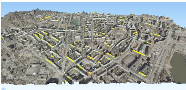
Figure 8. Visual exploration of potential solar panel locations on rooftops. Analysis is based on the use of DSM slope and aspect values, height differences between the DSM and the DTM, and building footprints.
