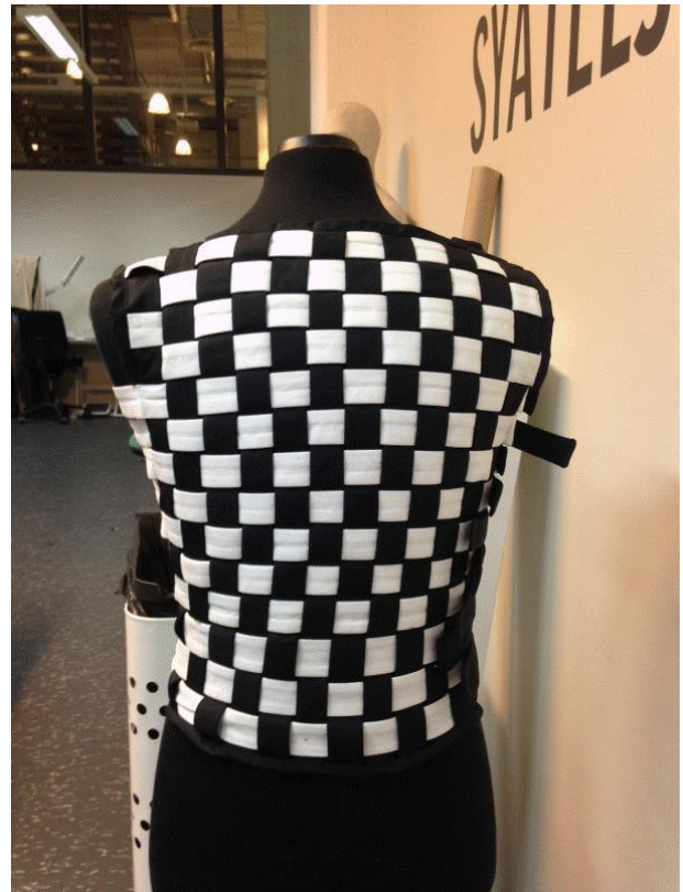
Figure 8. Back side of the textile testing device. Black squares belong to stripes in the vertical direction, white in the horizontal direction. Together a chessboard like appearance is formed. This results in an inherent matrix for specifying sign component positions.
