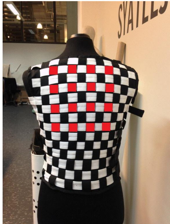
Figure 9. In-principle arrangement of 4 \times 4 actuators on the back of the smart vest. Actuators are to be placed beneath the red markers, towards the skin. The non-flat geometry of the human body that any haptic device has to handle is clearly visible.
