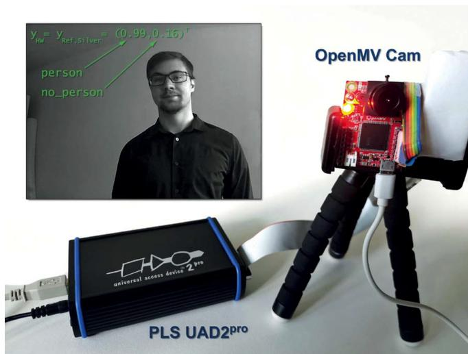
Figure 6. Hardware setup with OpenMV Cam H7 connected with the PLS UAD<sup>pro</sup> and an example of an input image for recognizing people. The reference models and hardware implementation certainly recognized the person (Ilkay Wunderlich) in the image.
