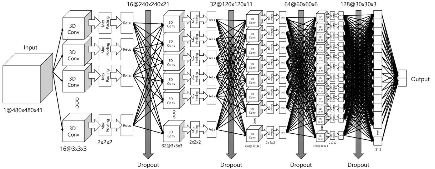
Figure 5. 3D Convolutional neural network structure
