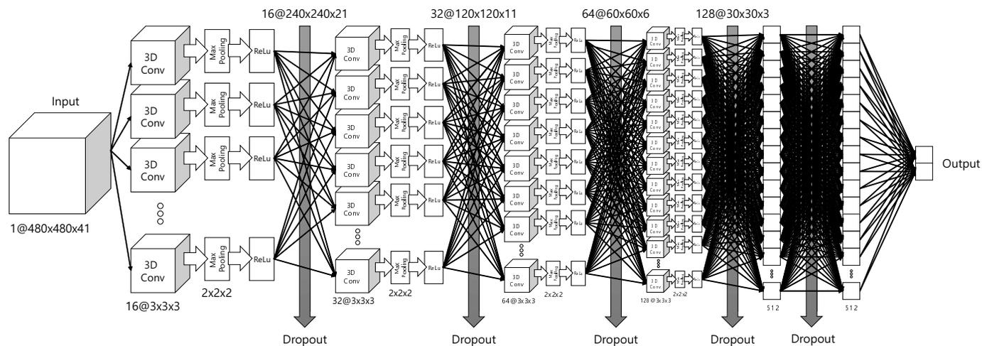
Figure 6. Extended 3D Convolutional neural network structure
