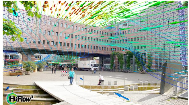
Figure 5. Enhanced augmented reality visualization
