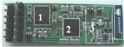
Figure 3. Redesigned module with added Power Amplifier (20mmx50mm)
