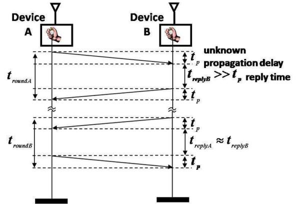
Figure 1. Symmetric Double Sided Two Way Ranging
