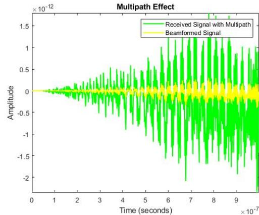
Figure 10. Multipath effect using 6 antennas.
