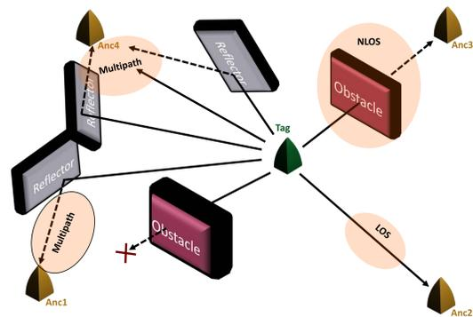
Figure 1. LOS and NLOS propagation of UWB signals [10].
