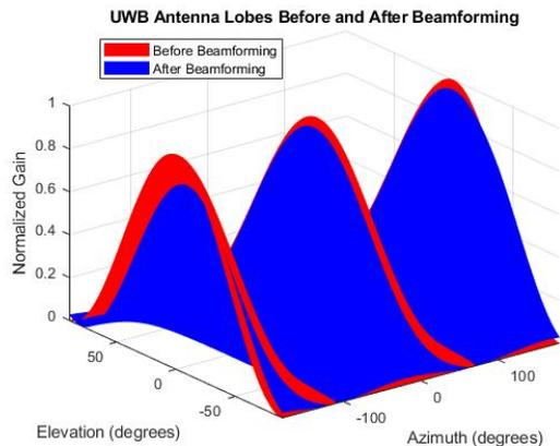
Figure 11. Beamformed and Non-Beamformed lobes.
