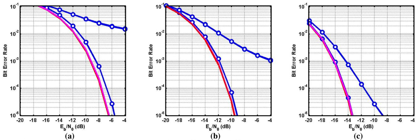
Figure 3. BER performances for SC/FDE-based MU-MIMO, with  $N_T = 10$ , and  $N_R = 10$  (a), 50 (b) or 100 (c), under reduced-complexity (I, II) and MMSE linear detection [ $1 \times N_R$  (single-path, multipath) reference BER performances are also included, and the five BER performances are ordered, from the worst to the best, as explained in section IV].
