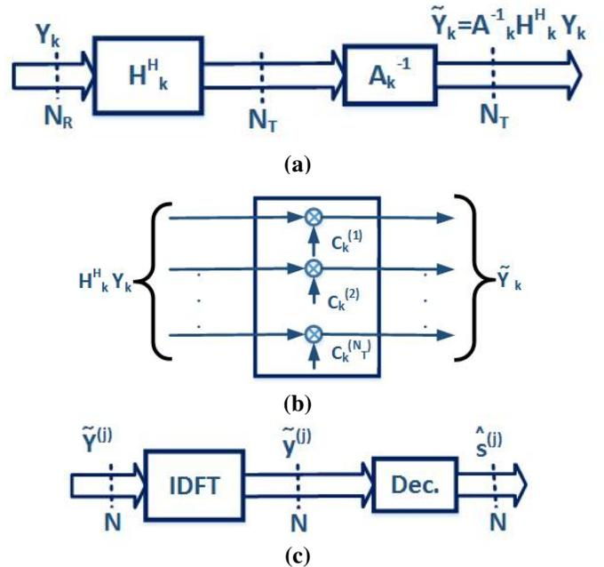
Figure 1. Linear, frequency-domain detection procedure ( $k = 0, 1, \dots, N - 1$ ) (a), reduced-complexity implementation regarding  $\mathbf{A}_k^{-1}$  (b) and time-domain decision procedure for user  $j$  ( $j = 1, 2, \dots, N_T$ ) (c).
