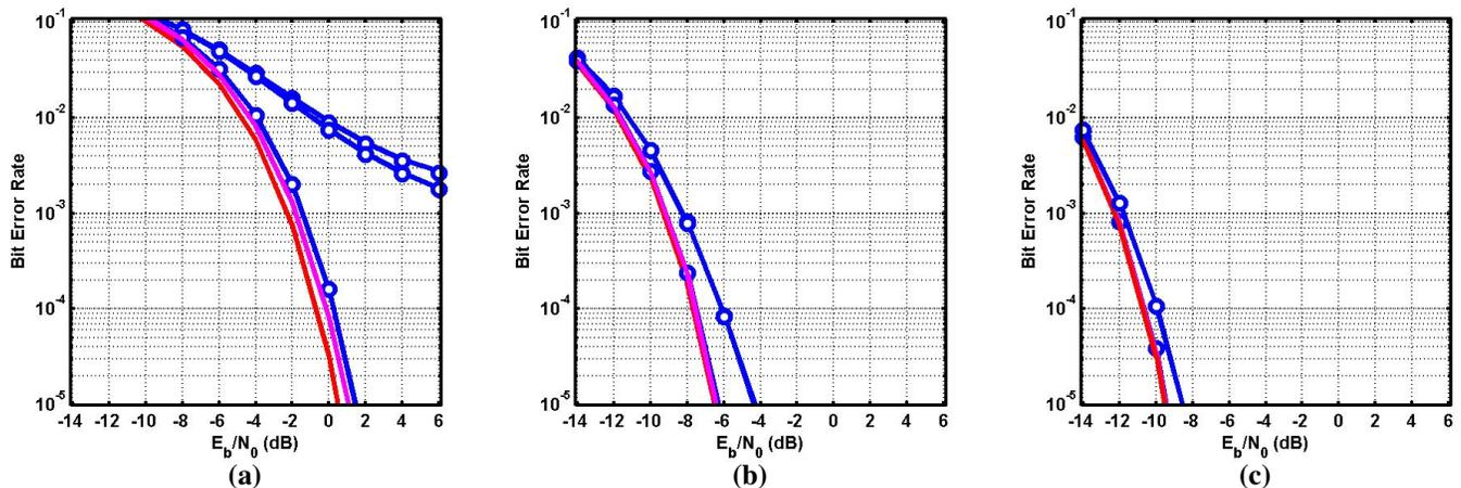
Figure 2. BER performances for SC/FDE-based MU-MIMO, with  $N_T = 2$ , and  $N_R = 10$  (a), 50 (b) or 100 (c), under reduced-complexity (I, II) and MMSE linear detection [ $1 \times N_R$  (single-path, multipath) reference BER performances are also included, and the five BER performances are ordered, from the worst to the best, as explained in section IV].
