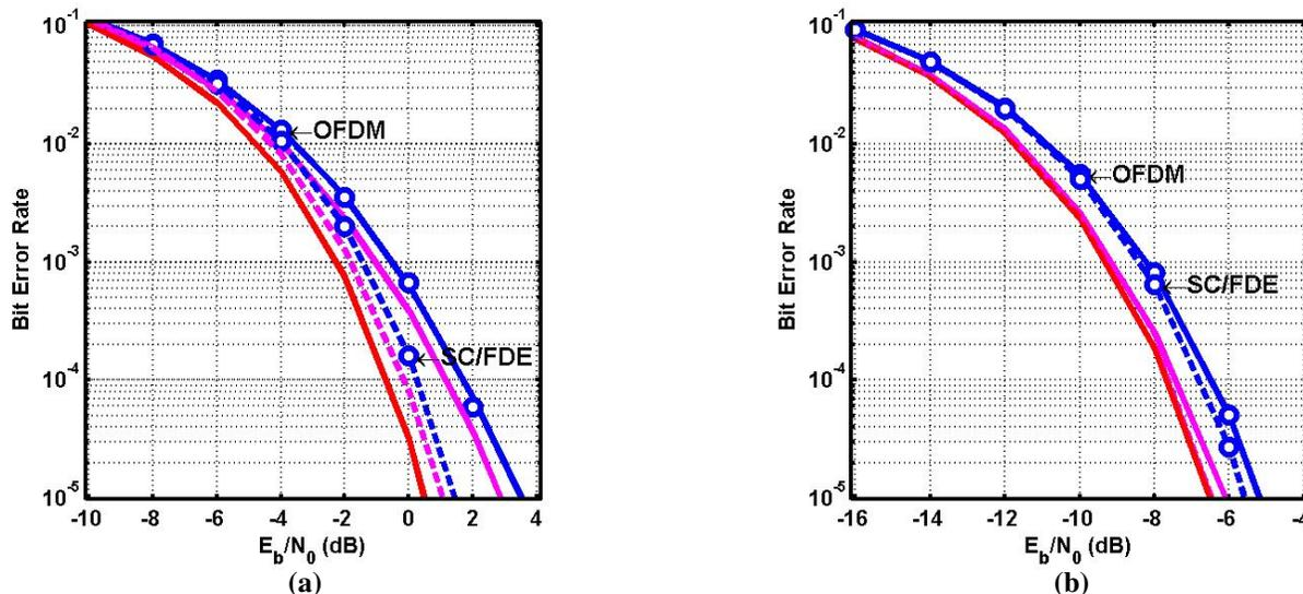
Figure 4. SC/FDE (dashed lines) vs OFDM (solid lines) BER performances, for  $2 \times 10$  (a) and  $10 \times 50$  (b), under strongly frequency-selective Rayleigh fading [SIMO  $1 \times N_R$  (multipath, single-path) reference performances are also included].
