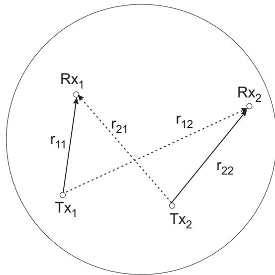
Fig. 1. Positions of communication devices inside a cell.
