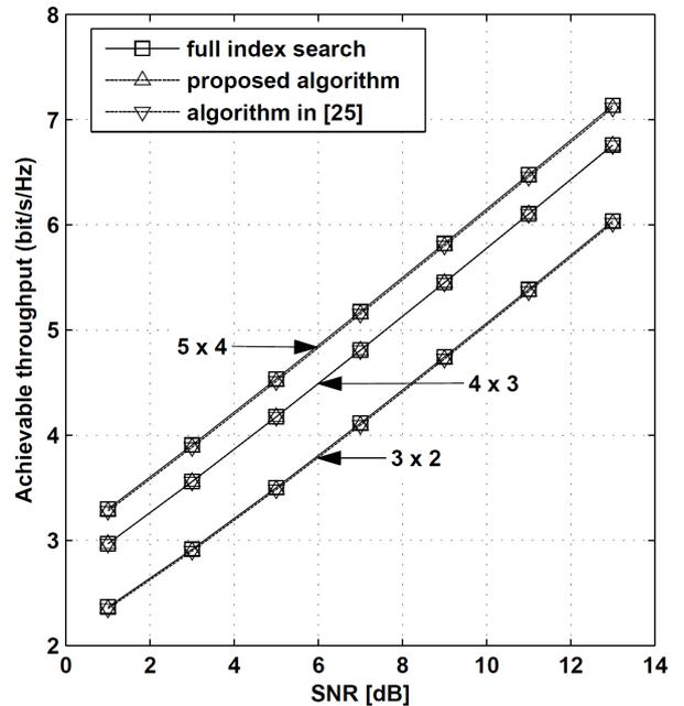
Figure 4. Throughput versus SNR when mobile speed is 50km/h.
