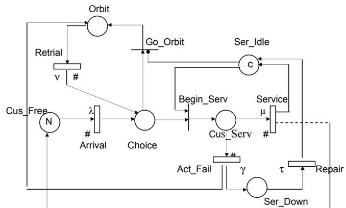
Figure 1. GSPN model of small cell wireless networks with retrials and active channels breakdowns
