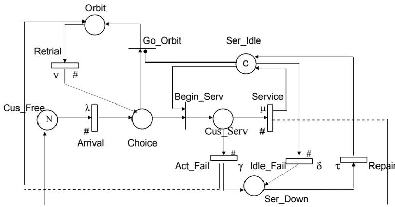
Figure 2. GSPN model of small cell wireless networks with retrials and dependent channels breakdowns
