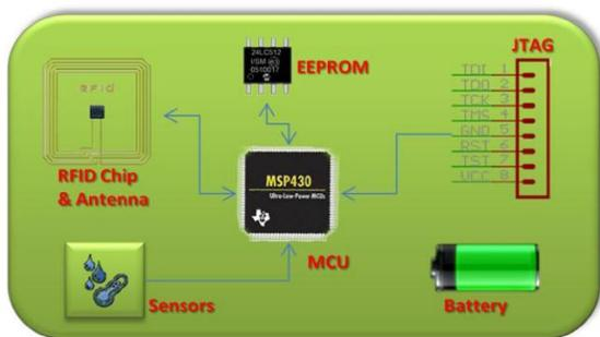
Figure 1 – SMART RFID Sensing Transponder architecture
