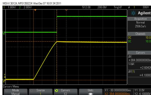
Figure 16: Case 1, All trimming bits are set to high state. TRIM<1:8>= High, TRIM<9:11>= High, Battery voltage = 4.1V, Charge Time: 384ms
