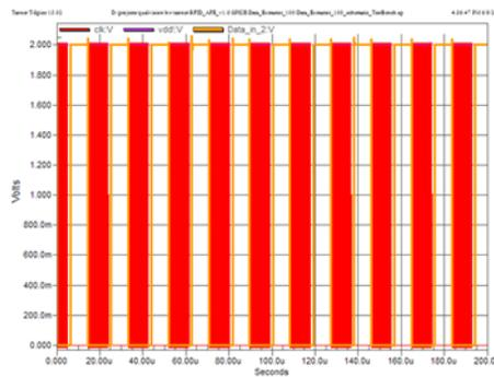
Figure 10 –100% OOK Modulation, Data extraction
