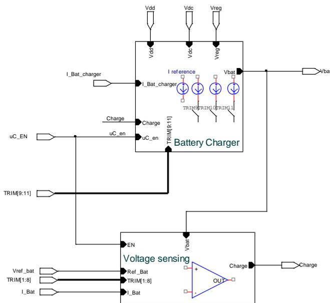
Figure 11 –Block diagram of the battery charger
