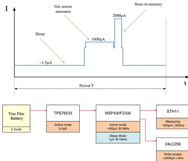
Figure 4 – Current consumption at different transponder operating steps
