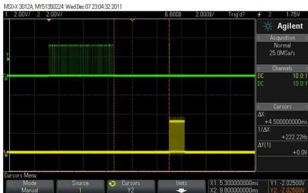
Figure 14 –Reader-Transponder communication: Write command
