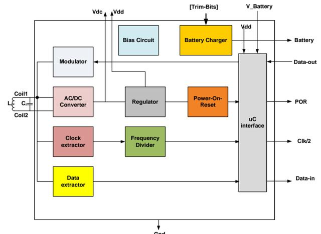
Figure 6 – RFID Analogue Front End Chip (AFE)
