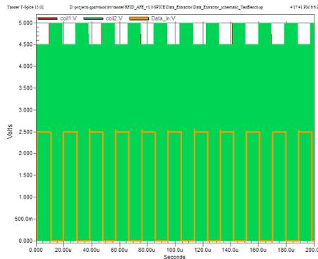
Figure 9 –10% OOK Modulation, Data extraction
