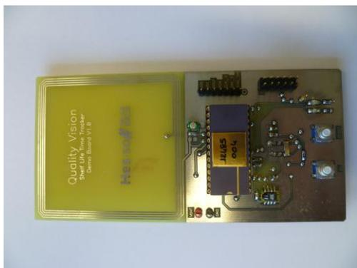
Figure 2 – SMART RFID Sensing Transponder prototype (Front view)
