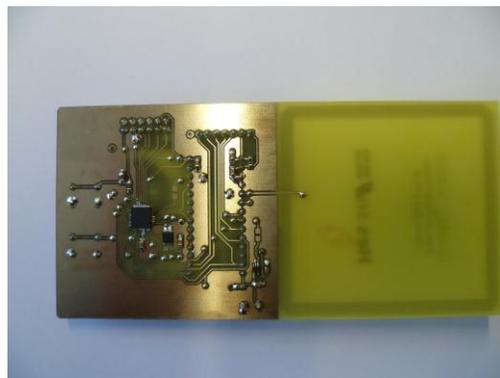
Figure 3 – SMART RFID Sensing Transponder prototype (Back view)
