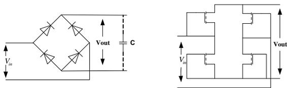
Figure 7 – Diode and MOS bridge rectifier
