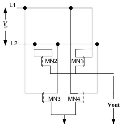
Figure 8 – Cross-connected MOS bridge rectifier
