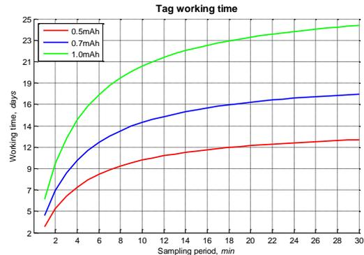
Figure 5 – Battery lifetime as function of the sampling period
