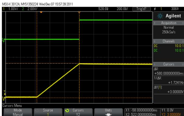
Figure 15: Case 1, All trimming bits are set to low state. TRIM<1:8>= Low, TRIM<9:11>= Low Battery voltage = 3.0V, Charge Time: 580ms
