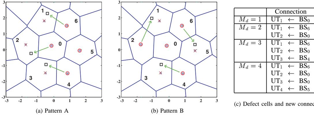
Figure 1. System model. Circles, cross marks, and box marks in (a) and (b) respectively denote working BSs, broken BSs, and active UTs in defect cells. Table (c) shows alternative BSs for UTs in defect cell (Pattern A), which is used in Section IV.
