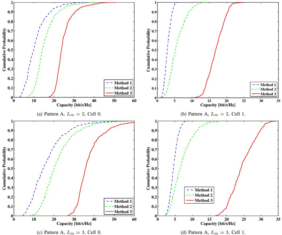
Figure 2. Distribution functions of sum capacity in two and three stream transmission for Patter A (SNR = 20dB).
