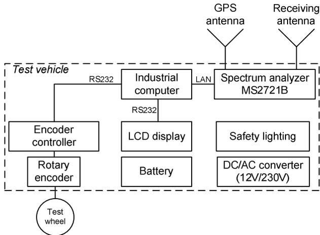
Figure 2. The block diagram of the mobile receiving section
