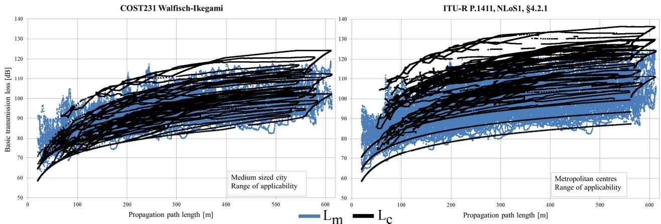
Figure 3. Basic transmission loss calculated on the basis of COST231 Walfisch-Ikegami model and ITU-R P.1411 model
