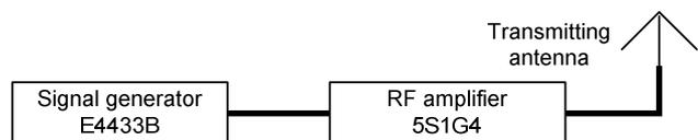
Figure 1. The block diagram of the fixed transmitting section
