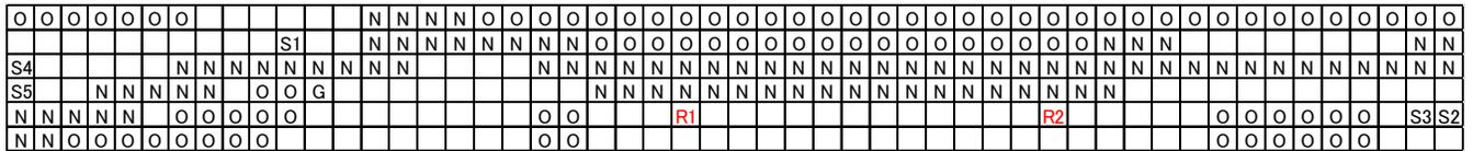
1cell = 10m × 10m, N: the relays installation impossible, O: the obstacles, S: the wireless sensors' location
