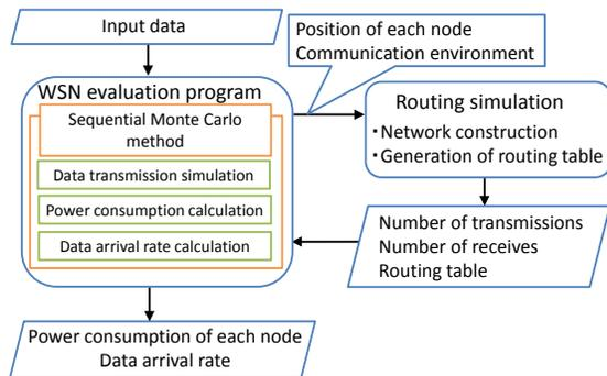
Figure 3. Configuration of WSN operation simulation
