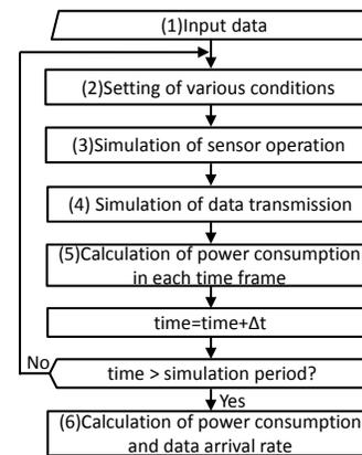
Figure 4. Flowchart of WSN operation simulation
