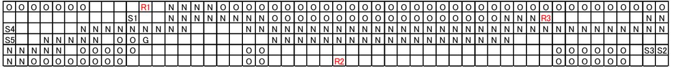
Figure 6. Calculation result of relay nodes placement by the proposed method (top view of monitoring area)
