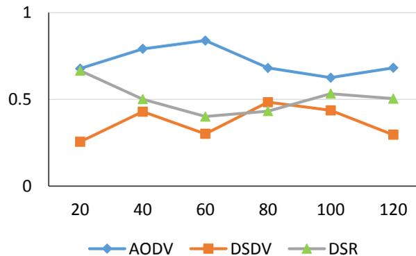
Figure 4. Packet delivery ratio vs number of nodes, DOS1.
