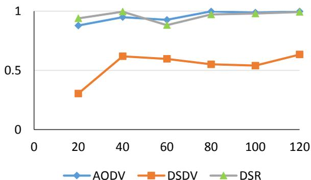
Figure 3. Packet delivery ratio vs number of nodes, no DOS.
