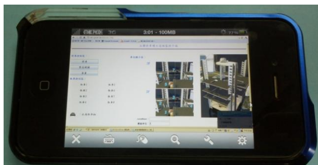
Figure 11. Remote management of the parking tower via a smart phone.
