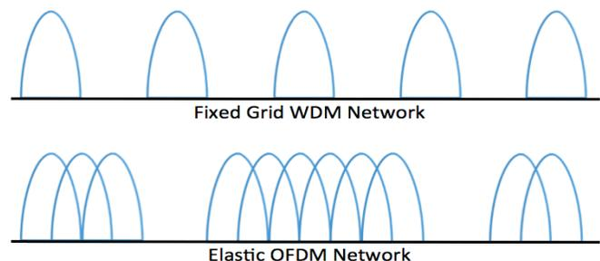
Figure 1. Comparing the spectrum of a WDM network with its fixed grid and that of an OFDM network with overlapping subcarriers.
