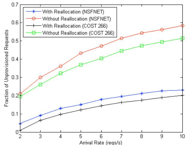
Figure 4. Comparing the routing and spectrum assignment algorithm for tight deadlines with and without the reallocation phase
