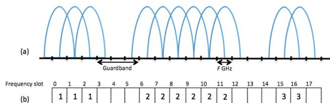
Figure 2. Relationship between the overlapping subcarriers (a) of several connections and an equivalent frequency slot model (b).
