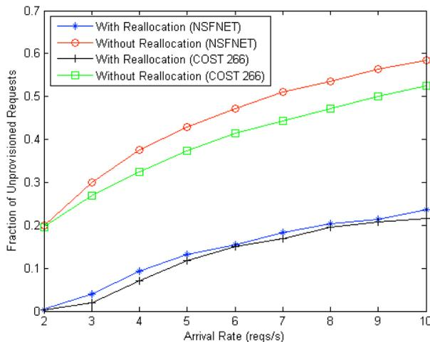
Figure 3. Comparing the routing and spectrum assignment algorithm with and without the reallocation phase
