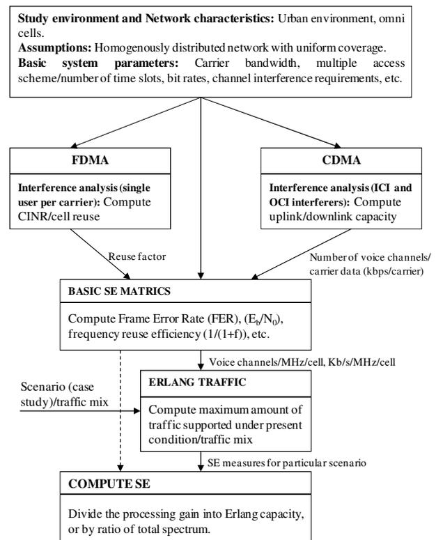
Figure 1. Spectral efficiency methodology
