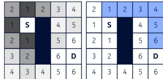
Figure 2. Lee's algorithm with occupied cells
