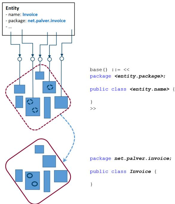
Figure 2. Instantiating a coding template with model parameters.
