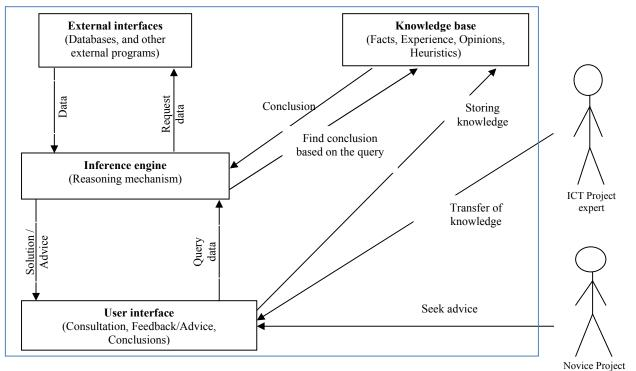
Figure 1. An architecture of the proposed expert system (adapted from [9][17])
