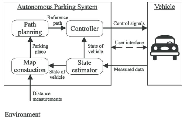
Figure 2. Components of the Parking Assist System [5]
