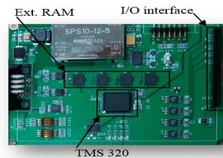
Figure 4. BEM consisting of a DSP processor
