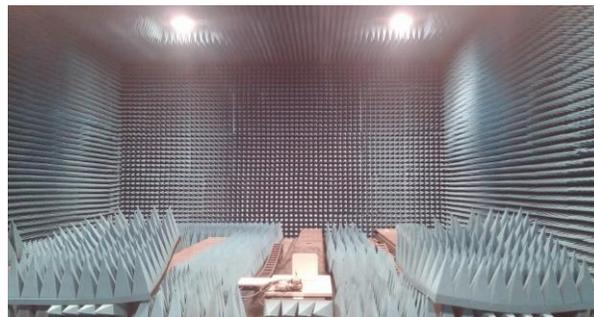
Figure 8. Used anechoic chamber for the performance measurement
