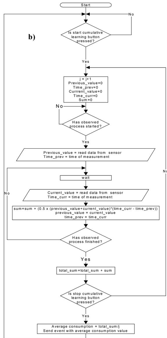
Figure 1. a) Range observation and b) process observation algorithm
