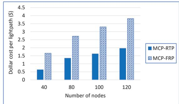
Figure 6. Comparison of electricity costs between MCP-FRP and MCP-RTP with different traffic loads for NSFNET
