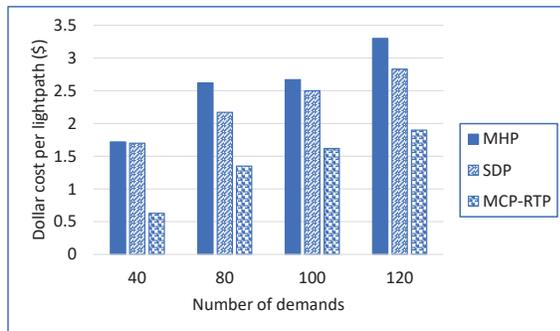
Figure 4. Comparison of electricity costs with different RWA approaches and different demands for NSFNET network
