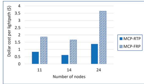
Figure 5. Comparison of electricity costs between MCP-FRP and MCP-RTP for different topologies and 40 demands
